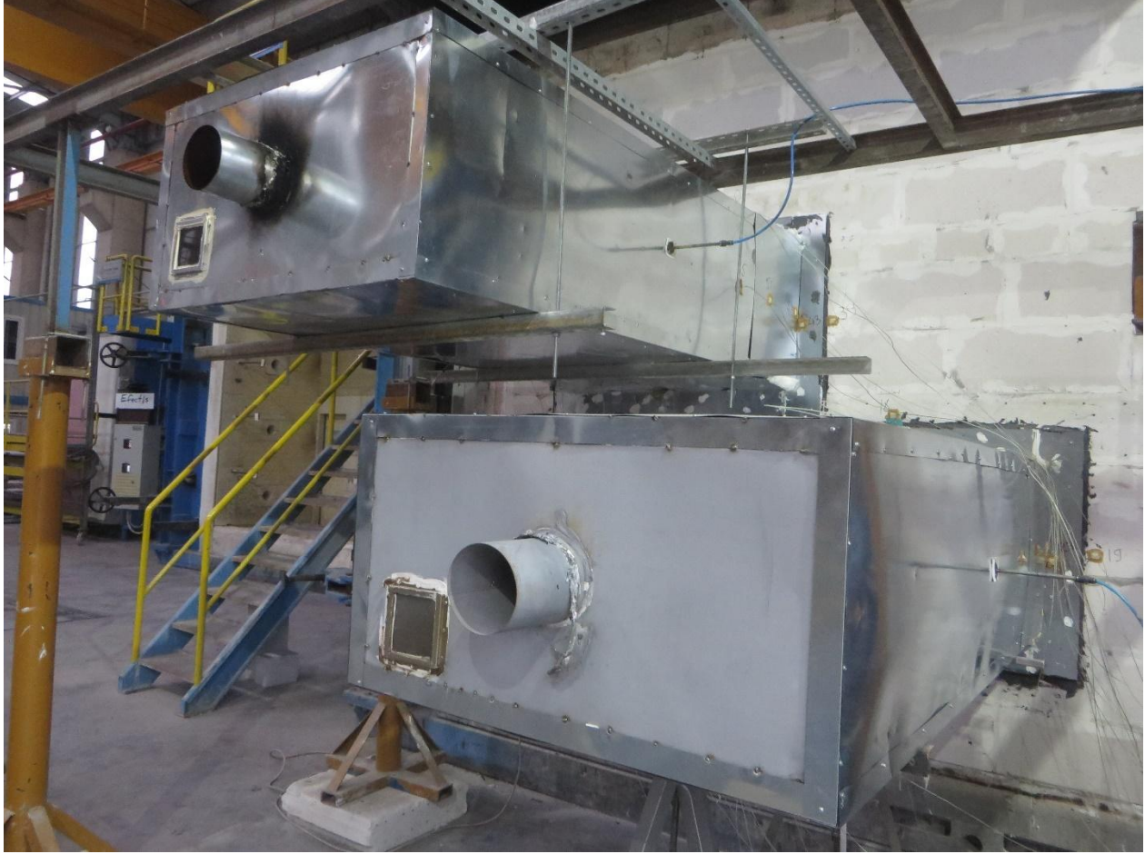
Photo C3: Unexposed side after the fire test
