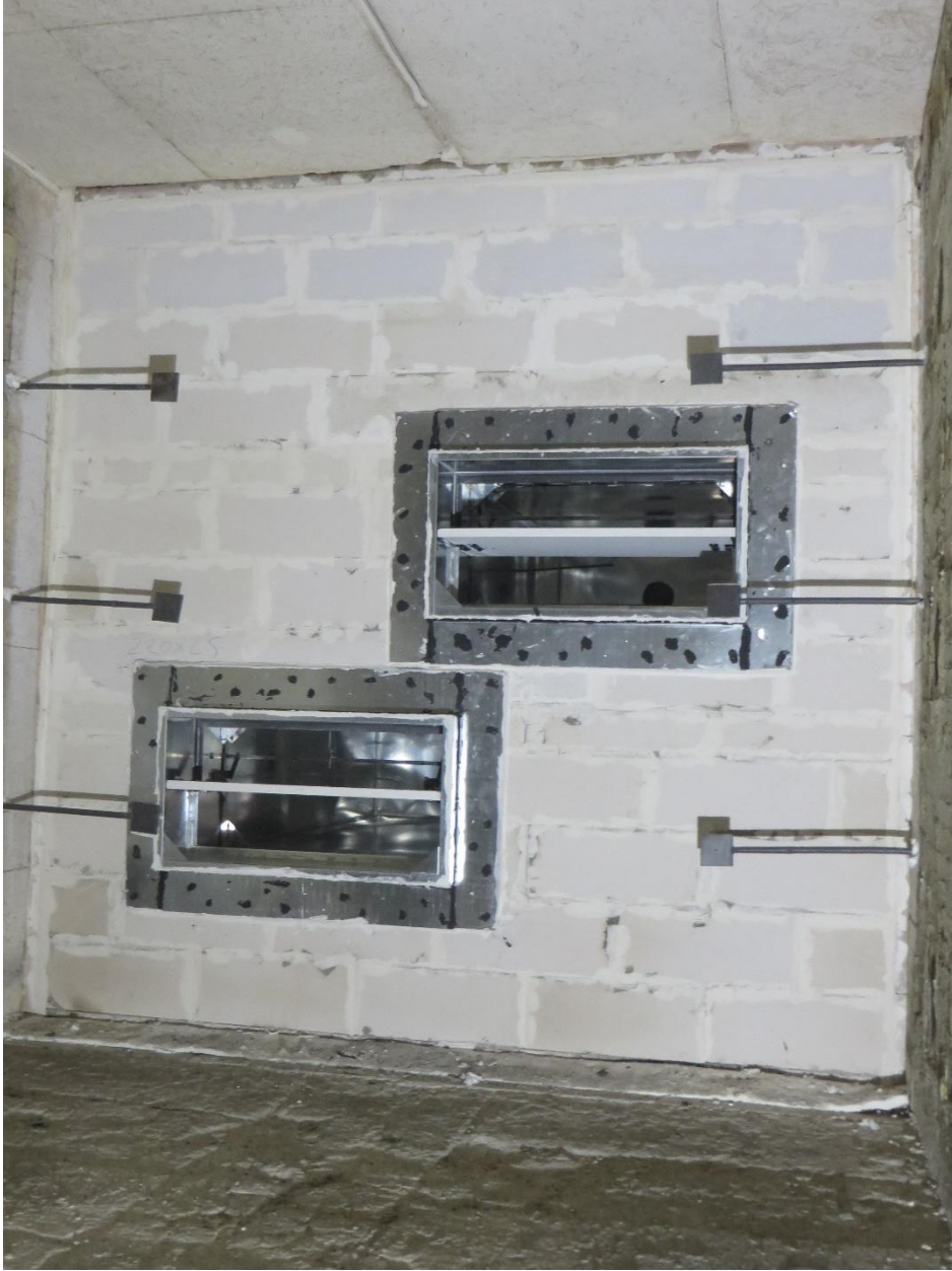
Photo C1: Exposed side of the specimen before the fire test
